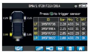
Activate and display sensor information for all OE TPMS sensors as well as most aftermarket TPMS sensors, including sensor ID, pressure, frequency, temperature, and battery status.
