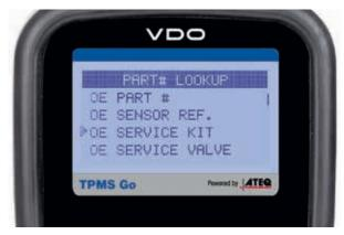
VDO TPMS Go guides you to compatible sensors and part numbers for any vehicle, and indicates the correct torque values.
