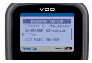
Quickly program aftermarket sensors, one wheel at a time. For relearning, use the VDO TPMS Go with a diagnostic scan tool or follow the vehicle's instructions for auto or manual relearn.
